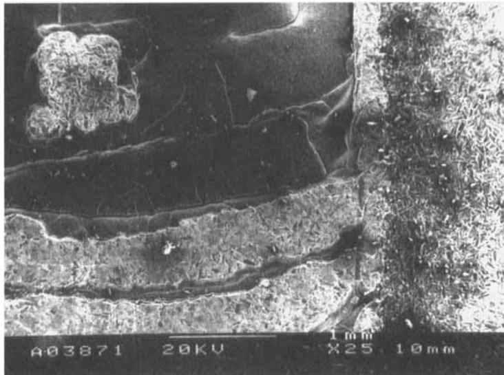
FIGURE 4 Scanning electron micrographs of the surfaces of (a) the substrate and (b) the rubber produced after peeling natural rubber compound 1A from steel with lower coating weight “Phosphate 2” treatment. Peel front advances from bottom to top.
